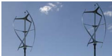
Helix wind turbines
